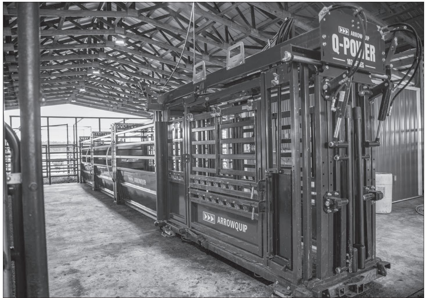
With this hydraulic cattle squeeze chute, Dr Jason Cater can examine his animals one by one, giving them the best care.
