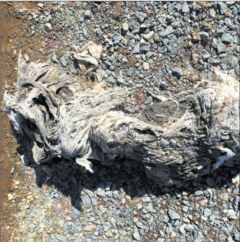
Items pictured above were pulled out of 8” sewer lines within the City of Monticello after being improperly disposed of. Above left is a 63” blanket, a pair of shorts, and a pair of denim jeans. Above right, a clump of “flushable” wipes are pictured.
