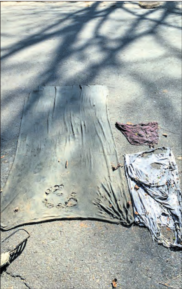
Items pictured above were pulled out of 8” sewer lines within the City of Monticello after being improperly disposed of. Above left is a 63” blanket, a pair of shorts, and a pair of denim jeans. Above right, a clump of “flushable” wipes are pictured.
