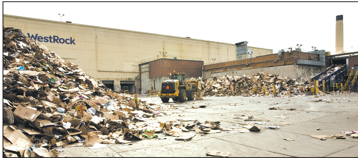
Cardboard placed in recycling bins is picked up by Eureka Recycling and sorted at their NE Minneapolis facility. It ends up here at WestRock in the Midway neighborhood, where it is remade into one of two types of recycled paper. (Photo by Margie O'Loughlin)
