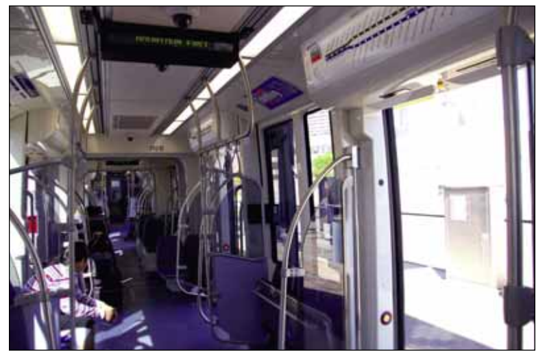
Inside the train: Priority seating for persons with disabilities is situated next to the door. Bikes can be brought on board and parked vertically, held upright by a hook. Route maps are posted above each door. (photo by Jill Boogren)
