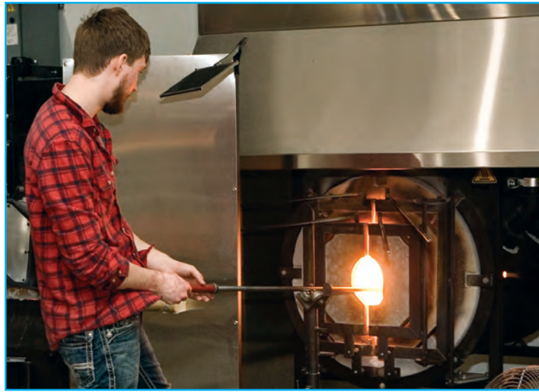
Borkhuis re-heated the glass he was working in what glass blowers affectionately call, "The Glory Hole." The temperature here is 100 degrees higher than the furnace. (Photo by Margie O'Loughlin)
