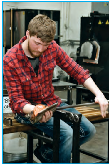
Bryce Borkhuis, studio manager, shaped molten glass with a hot pad made from newspaper pages. Glass artists don't wear gloves, even though they're working with a material that has been heated to more than 2,000 degrees. (Photo by Margie O'Loughlin)
