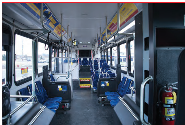
The 40-foot Gillig model buses look significantly different than regular-route buses. Passengers will be able to get on and off faster, thanks to low-floor buses and raised curbs at stations, plus wider bus doors and boarding from the front and back. (Photos submitted)
