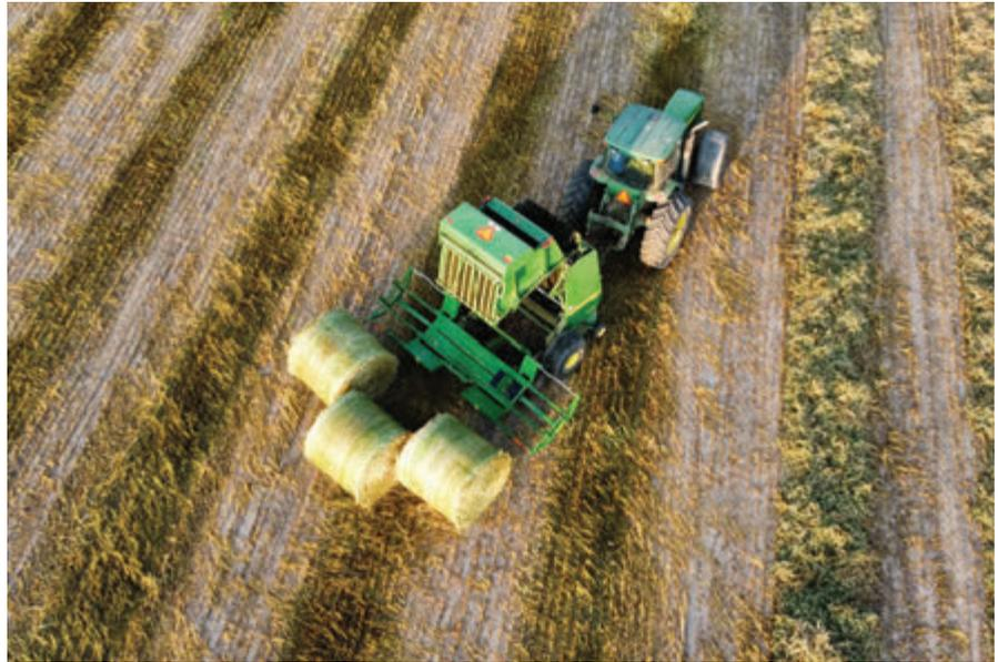
The 521R and 421R Bale Accumulator allow round baler operators to carry multiple bales of hay.
