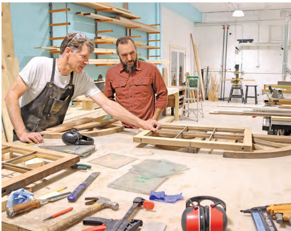
Woodworker Bill Dossett (left) and Joe Hayes look over a set of windows being restored. According to Dossett, the dust collection system in the new building is an upgrade that has made a big difference for staff. Plus there's a room just for planing. (Photo by Tesha M. Christensen)
