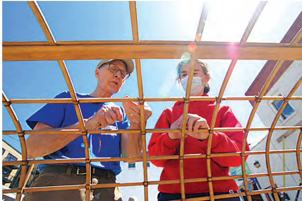
David Walcher of Urban Boatbuilders instructs Masyn May to lace ribs to the frame of a canoe. (Photo by Terry Faust)
