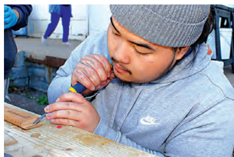
Htoonoh chiseles grooves in cross-bar canoe supports. (Photo by Terry Faust)
