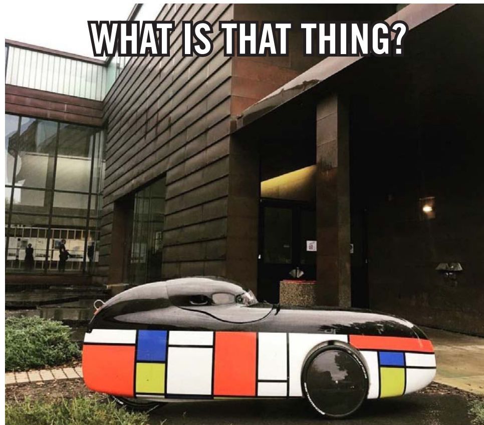
It's Don McCall's velomobile – a three-wheeled bicycle imported from Holland. McCall, who lives in Como, can reach 25 miles an hour in his velomobile on a good day.
