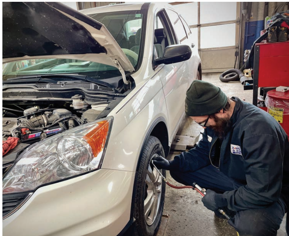
Technician Paul Edgar checks the tire pressure after testing the battery. "We have seen a large increase of people driving less during the pandemic. Letting your car sit for longer periods of time can cause it to fail. A battery not getting fully charged regularly can cause it to fail also." (Photo by Susan Schaefer)
