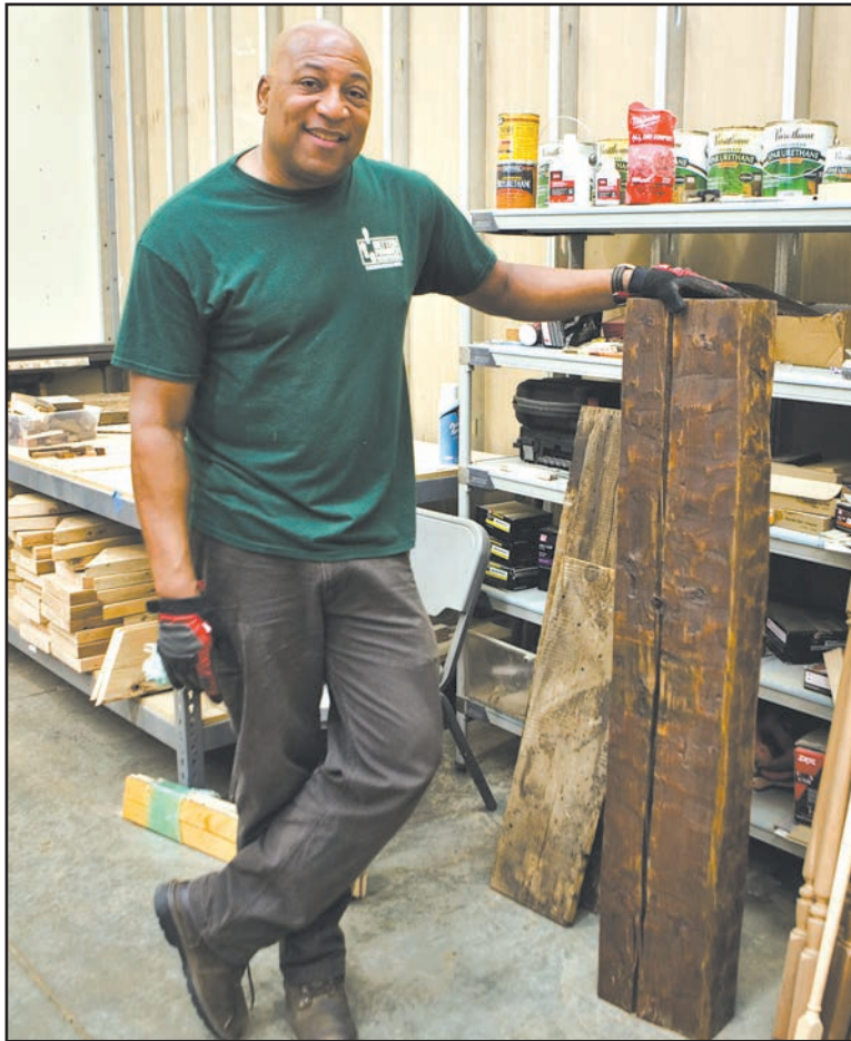
According to Jason Allen, pieces like this solid oak timber can't be bought at stores selling new wood products. The timber is 100+ years old, meaning that the wood grain is tighter, and the pitch content is high (making it naturally insect and rot resistant). (Photo by Margie O'Loughlin)
