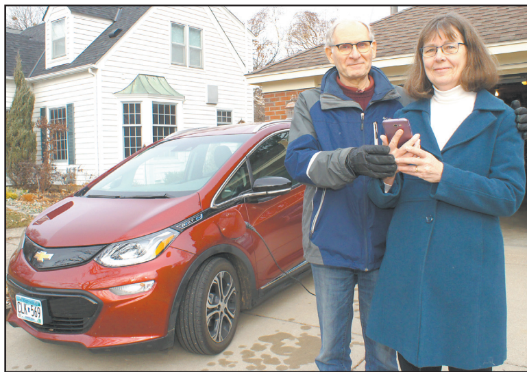
Rod Johnson and Kathy Hollander love their Chevy Bolt. The charging unit plugs into a standard 110 volt wall outlet, and then the charging plug fits into a port on the outside of the car. Using the ChargePoint app, users can monitor the Bolt's charging progress while away from the car. The Bolt can go about 240 miles on a full charge. (Photos by Terry Faust)
