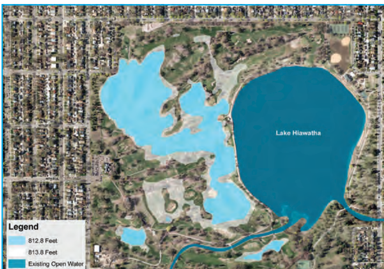
This graph shows the elevations of the land and water of Lake Hiawatha. The dark blue shows existing open water, while the light blue shows the area that falls below the 812.8 elevation of the lake, and would be under water if the pumping were to stop altogether. The white area shows the portion of the golf course that is at 813.8. (Photo submitted)
