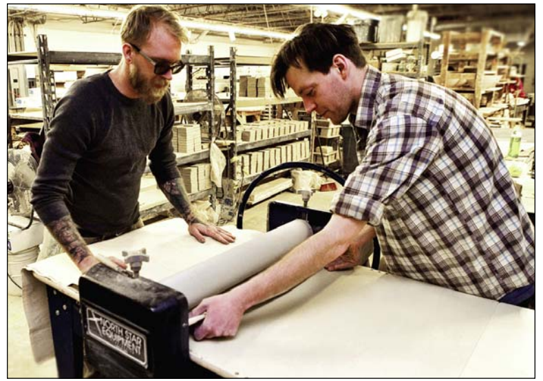
Using the slab roller to prepare clay for tile production. (Photo by Margie O'Loughlin)
