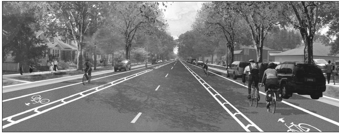
A view of what the reconstructed Minnehaha Ave. will look like. The roadway will include "buffered" on-street bike lanes (shown above) over fully "protected" bike lanes, which are separated from traffic by a curb, parked cars, or other physical barrier. (Image prepared by LHB and SRF on behalf of Hennepin County)
