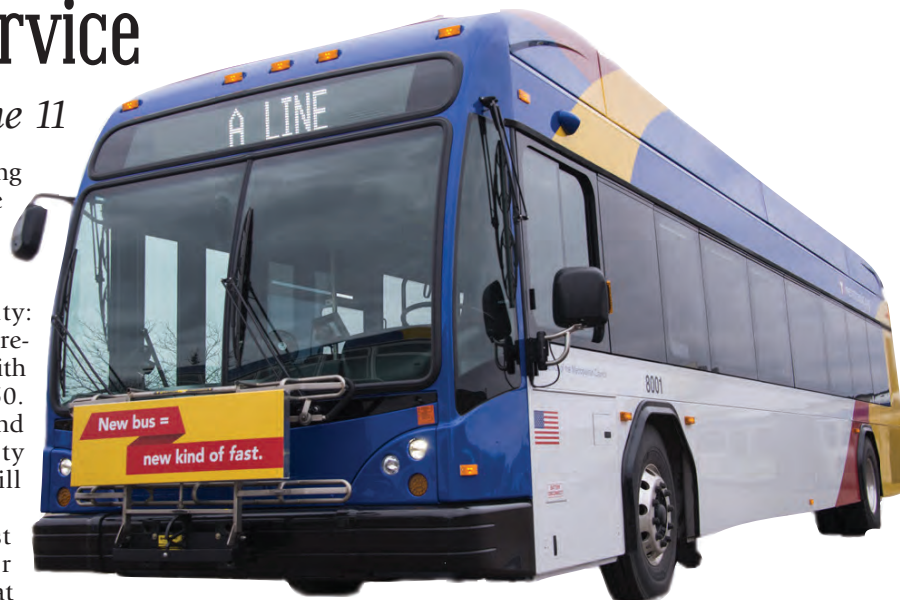
The 40-foot Gillig model buses look significantly different than regular-route buses. Passengers will be able to get on and off faster, thanks to low-floor buses and raised curbs at stations, plus wider bus doors and boarding from the front and back. (Photos submitted)
