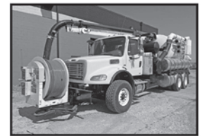
EK8700 '11 Freightliner Biz Class M2 sewer jetter truck
