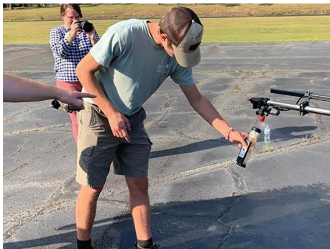
SPENCER LAWRENCE RECEIVES TRAINING ON USING A SPOT-ON SPRAYER CALIBRATOR TO CHECK THE FLOW RATE OF INDIVIDUAL SPRAYER NOZZLES FOR MORE EFFECTIVE PESTICIDE USAGE
