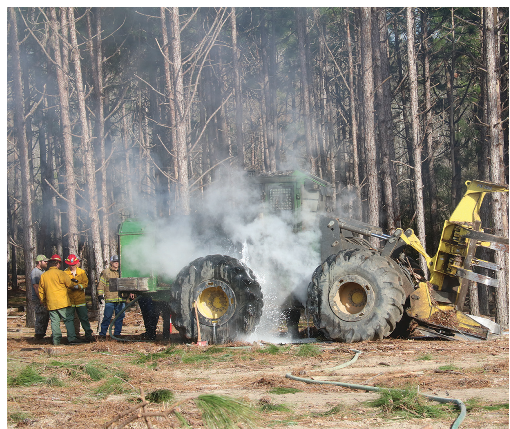
FOAM BEING APPLIED TO BURNING HYDRAULIC FLUID
