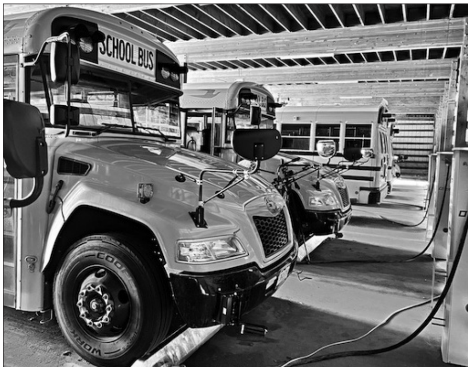
EV buses charging in a facility
